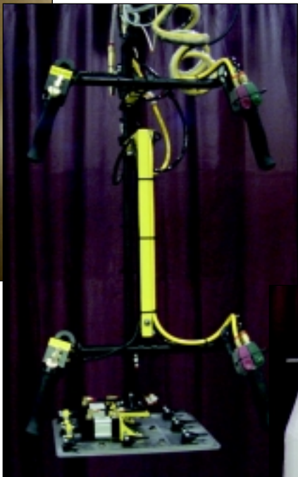
The spool handling device shown here used by a major pharmaceutical products manufacturer, has Dual Controls. The spools are stacked 3-high in a box and the Dual Controls enable the operator to pick up spools without bending.
