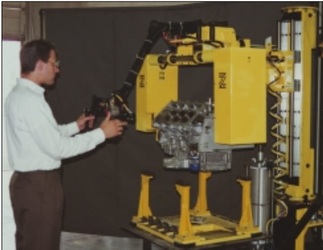
Air clamp handling device for engine rollover
