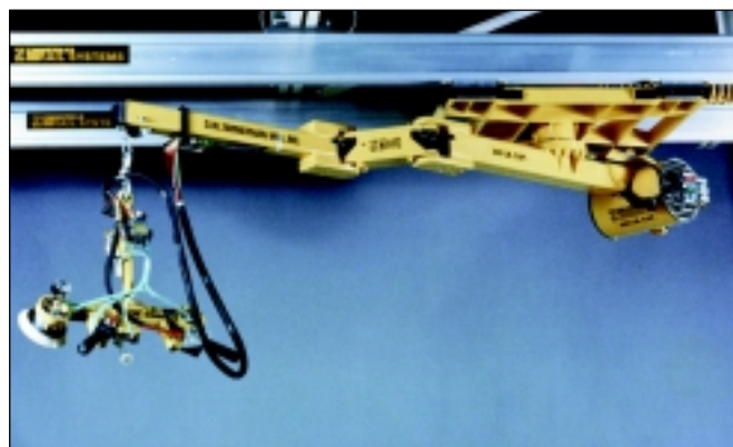
700 C Arm (carriage mount) shown with optional end effector
