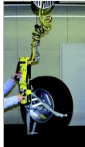
Tire handling device with 90 degree manual rotate.
